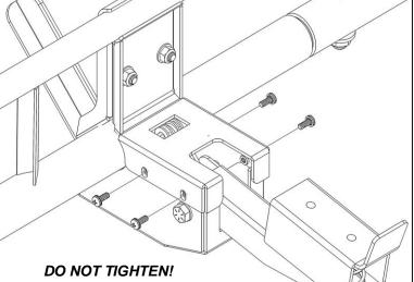
• TIGHTEN 5/16" hex head bolts from Step 3, THEN tighten remaining hardware.
