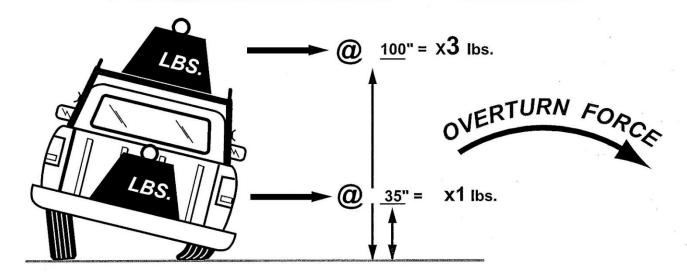
WEIGHT CARRIED ABOVE THE FLOOR OF THE TRUCK BED (E.G., ON AN OVERHEAD TRUCK RACK) WILL SIGNIFICANTLY INCREASE THE VEHICLE'S TENDENCY TO OVERTURN. ALWAYS KEEP HEAVY LOADS EVENLY DISTRIBUTED AND AS LOW AS POSSIBLE. IT IS IMPORTANT TO NOTE THAT THE HOLMAN RACK LOAD BEARING CAPACITY MAY BE GREATER THAN YOUR TRUCK'S GAWR OR GVWR CAPACITY AND IS PROBABLY GREATER THAN THE WEIGHT THAT CAN BE SAFELY CARRIED OVERHEAD. ALWAYS RETIGHTEN ALL BOLTS AFTER FIRST USE. REGULARLY CHECK BOLTS FOR TIGHTNESS.
