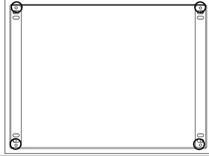
Place Kargo Case holder in desired position on bottom of DCU shelf. The small flange on the Kargo Case holder goes towards the front, where the case will be accessed.
