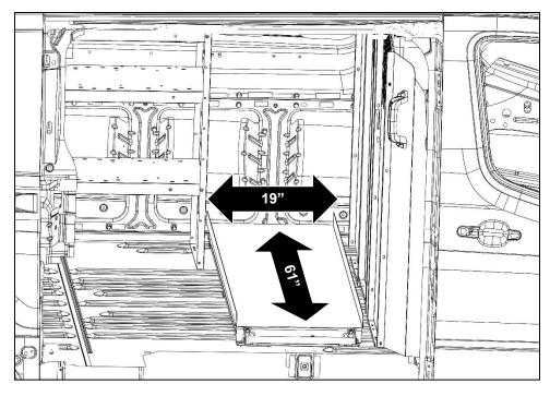
• Position mount assembly in desired location in vehicle. Be sure to allow enough clearance in front of slide rails to close van side door.
