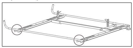
Mount the tube assembly to the bows using 5/16" x 2" carriage bolts, 5/16" flat washers and 5/16" lock nuts.
