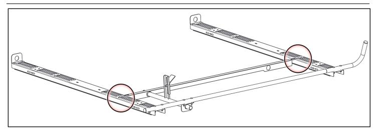
• Attach the long angle bracket to both bows in the orientation shown using 3/8" x 1" carriage bolts, 3/8" flat washers and 3/8" lock nuts.
