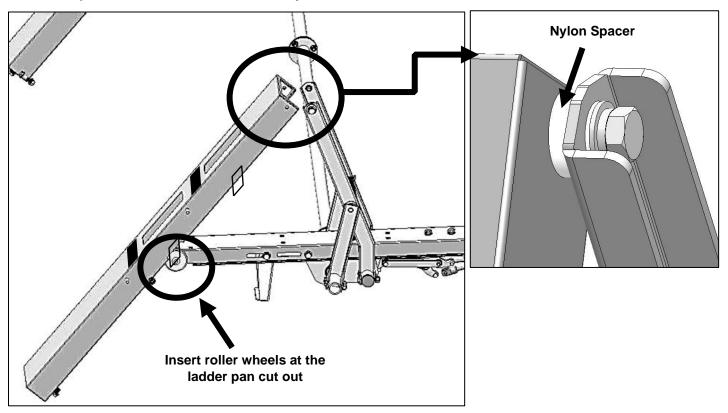
Caution: Make sure the nylon spacer is sandwiched between the arm and ladder Pan, and lock washer or lock nut is used on this assembly.
