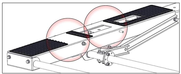
• Bolt into place using the pre-assembled hardware on both front and rear pan.
