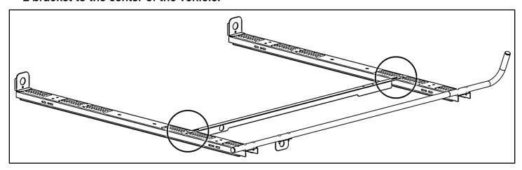
• Insert the plastic bushings into the clamp and lock L bracket and angle bracket installed in Step 5, with flange towards each other and to the inside as shown.
