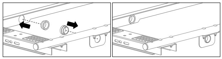
• Insert clamp tube into both plastic bushings in the orientation shown. Be sure to install the bushings in an orientation so they CANNOT fall out.
