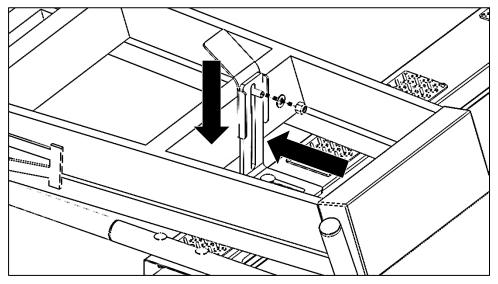
Press the ladder towards the rear and the angle pads against the ladder rung, tighten the bolt securing the front ladder stop to the front bow.
