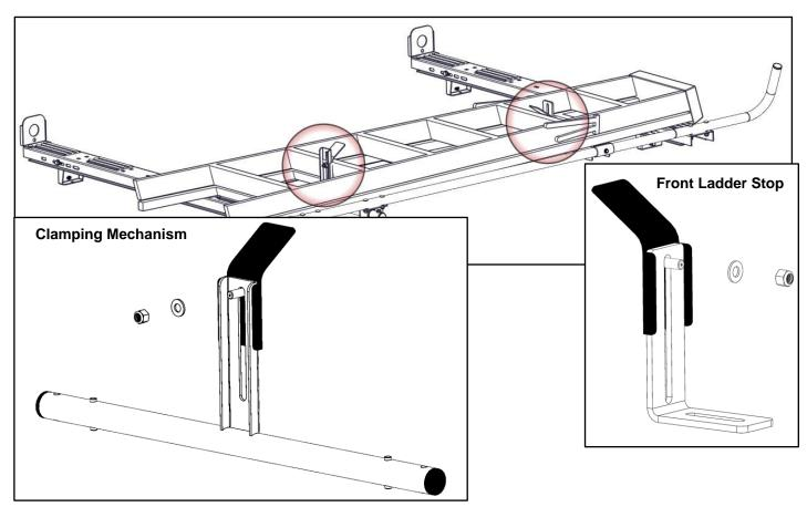
Loosen the bolt that secures the front ladder stop to the cross member.
